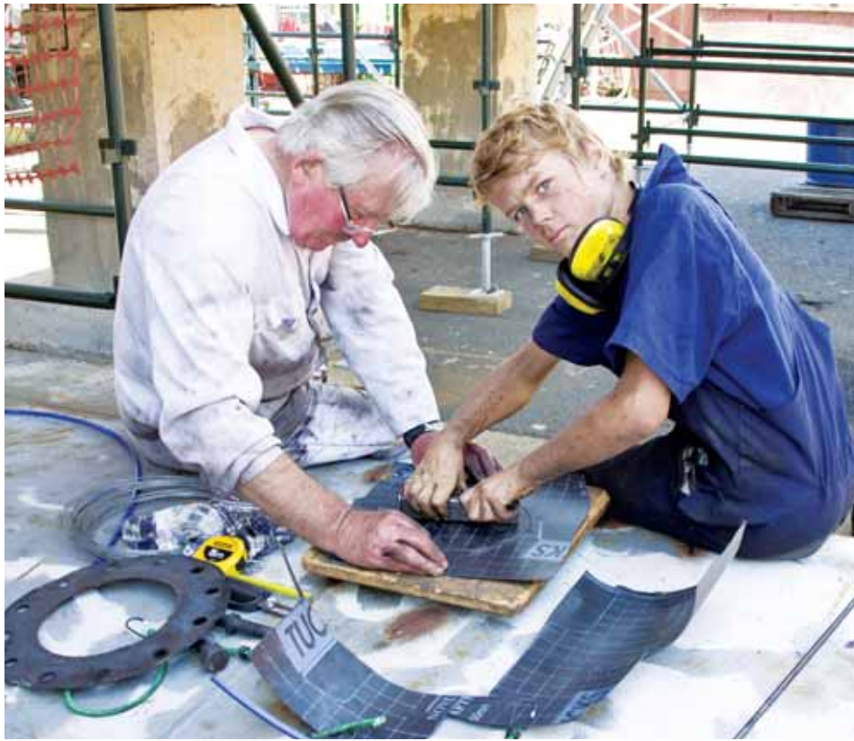
Marine engineer John Rogers shows Charlie how to cut a gasket.
